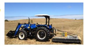
New Holland TT75 (75hp) Tractor with 6" Slasher and 4 in 1 Loader Bucket
