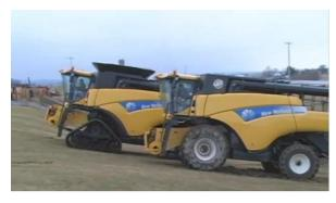
New Holland Header owners can harvest in wet conditions without tearing up their fields with New Holland's SmartTrax, now available for CR Series combine models. The rugged, triangular SmartTrax track system replaces the wheels on the combine's front axle. The proven design uses two 36-inch wide rubber tracks, which reduce ground pressure by as much as 60 percent compared to dual drive tires, with only minimal soil disturbance and less soil.
