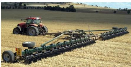
40FT MACHINE WITH COULTER SPACING AT 130MM
